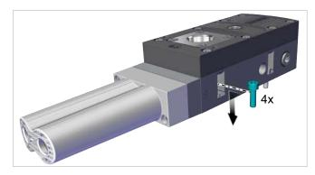
Use the supplied M5 screws (4x) to secure the ejector to a suitable mounting with a max. tightening torque of 5 Nm.
