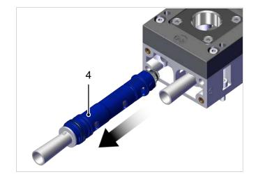
2. Pull the ejector module (4) out of the borehole.
