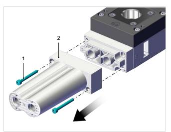
2. Fasten the new silencer with the two new screws using a tightening torque of 2 Nm.
